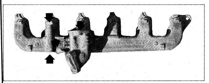
because of their greater heat dissipation—so even for looks they're not worth it. The stock cast-iron exhaust manifold retains the heat, operating the turbo more efficiently. In our case, the stock outlet on the exhaust manifold was cut off and Ak arcwelded on a 4-bolt flange plate to bolt the turbo's exhaust housing to. If you plan on building such a setup yourself, remember that special cast-iron welding rod must be used.
